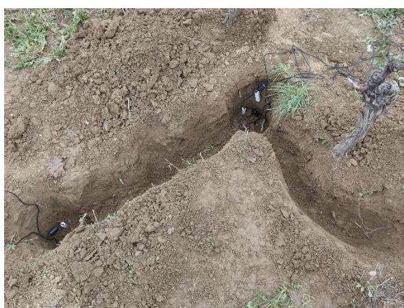
Fig. 2 Use of capacitive probe to study water behaviour in the soil – OG OFIVO
