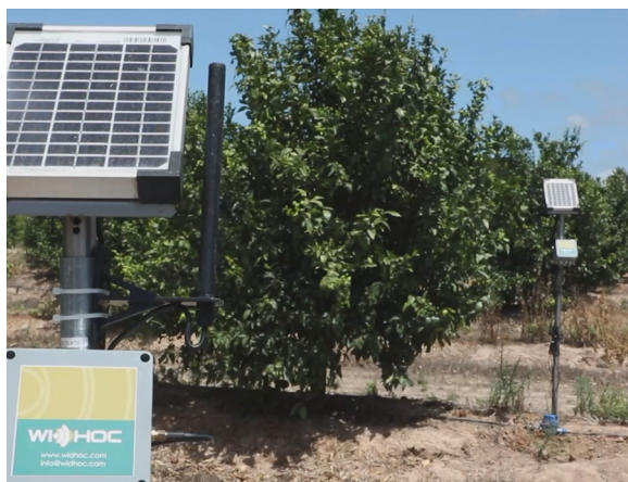
Fig. 10. Capacitance probe on an citrus plantation, similar to the probes used in OG GO AVOCADO
