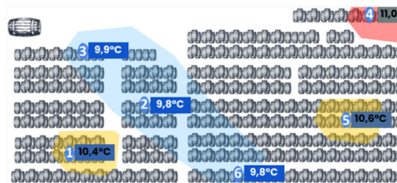
Fig. 3. Using cellular mapping to identify micro-climates to optimise evaporation loss and save on energy use 17
