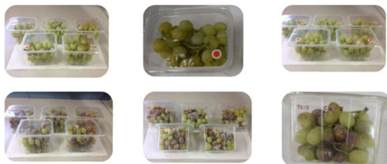
Fig. 2. Bunches of Superior Seedless grapes on day 15, packaged with BlowDevice® (above) and with a micro hole (below) 8
