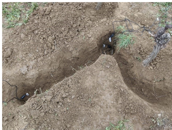
Fig. 4. Use of capacitive probe to study water behaviour in the soil – OG OFIVO
