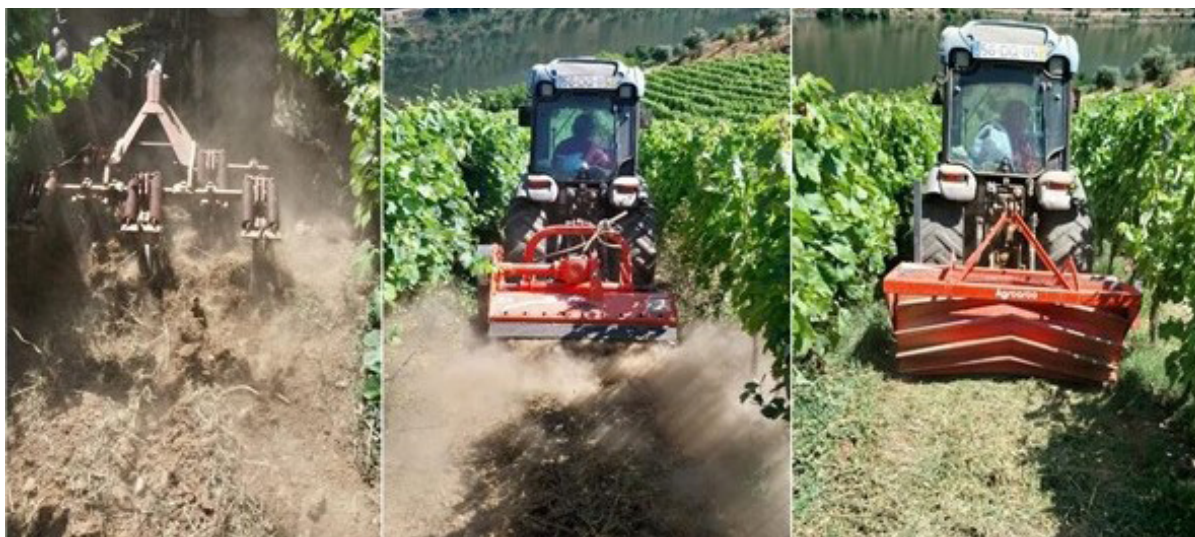
Fig. 5. a) TILL– tilled soil, b) MOW – mowed vegetation, c) ROLL – rolled vegetation 23
