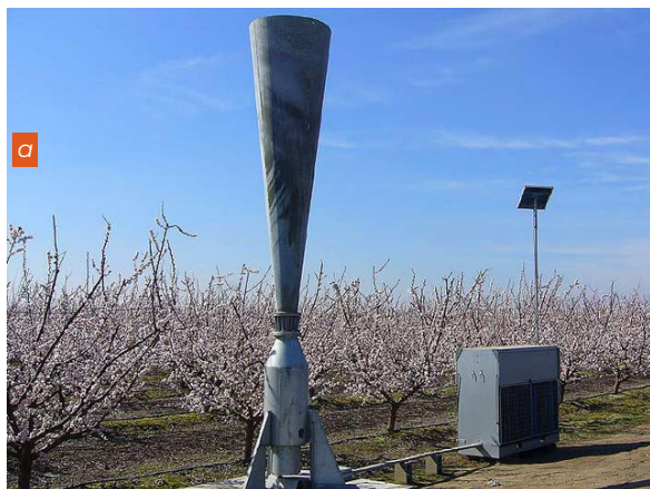
Fig. 7. a) Hail cannon 13 and b) operational diagram 14
