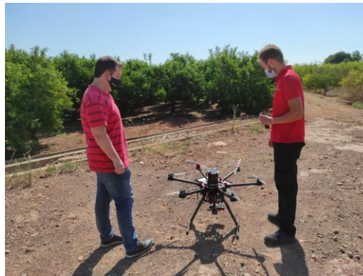
Picture 3. Drone equipped with thermographic cameras
