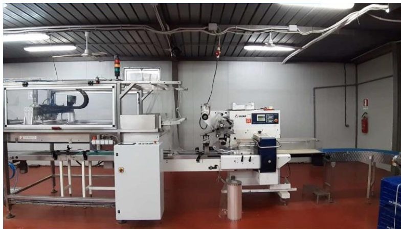
Figure 2. Flow pack machine for inserting BlowDevice® in film packaging at the Romanazzi company
